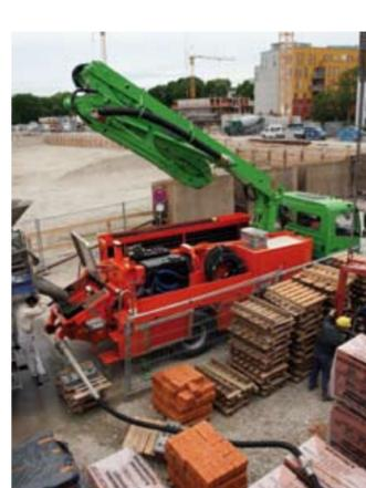
The flexible Z roll and fold 4-arm boom is able to access the smallest of openings in a building without the slightest effort. With hose extensions – attached to the boom end or directly onto the hopper outlet – the M 20-4 is the master of renovation work. (Illustrations show some optional equipment.)
